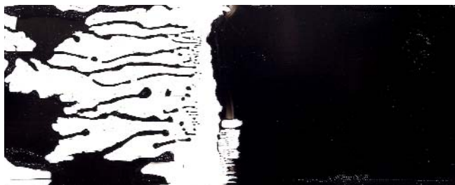
Figure 1: Paint finish on a contaminated substrate
