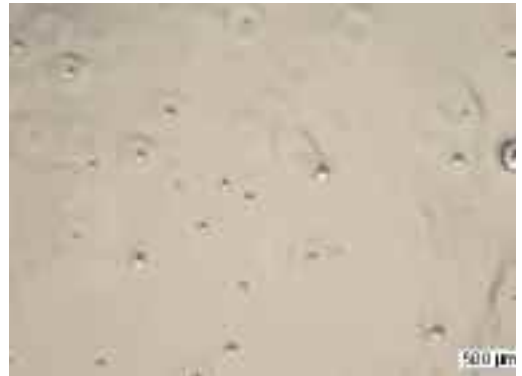
Figure 6: Microscopic view on waterbased Acrylic wood coating Above: With 0.3% Tego Airex 902 W Below: 0.3% Tego Airex 902 W + 0.3% Tego Twin 4100
